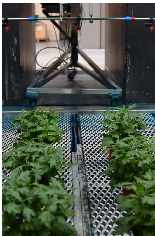
Figure 1. Six plants underneath the three-nozzle boom on the track sprayer
